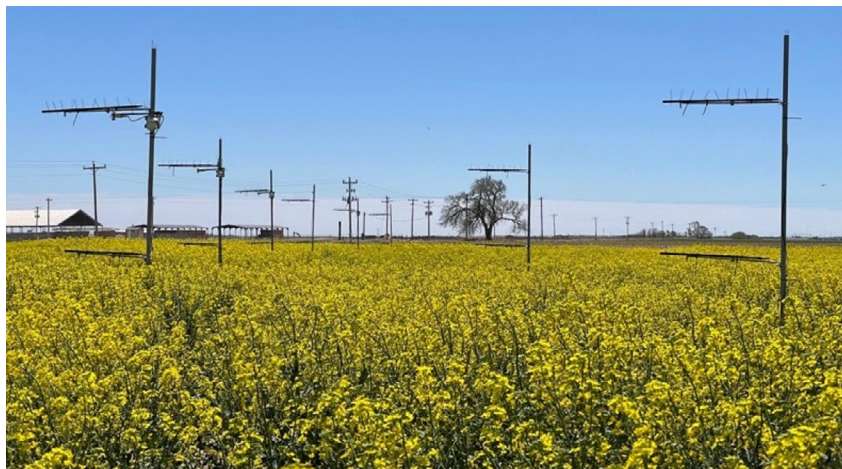
Line quantum sensors installed at different heights in winter canola field during peak flowering stage at Clovis, NM.
