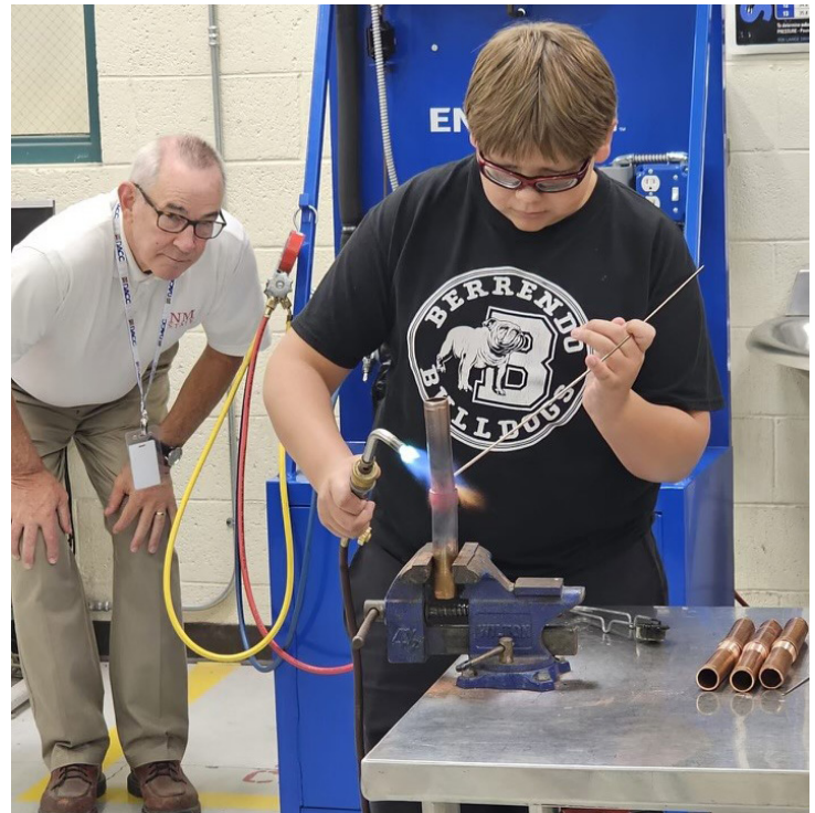
A middle school student brazes copper pipe during a hands-on visit to the DACC HVAC R program as part of the Aggie Next Step College Experience.
